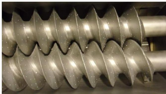
**Figure 3: Screw shafts of the heat exchange [4]**
